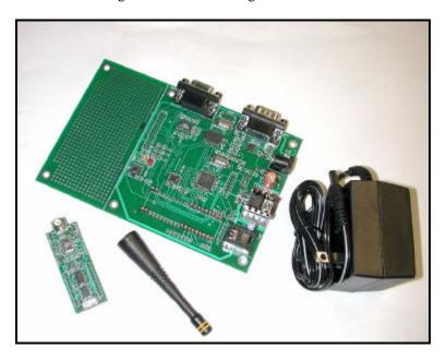
Transmitting and receiving data at 20kbps in the unlicensed 900MHz band, the **CANRF** will connect CAN nodes up to 250' apart. Power output is set at 0.25mW into 50 ohms (-1.25dBm) but can be adjusted up to 0.75mW if an inefficient antenna keeps the signal down below the FCC Part 15 regulations.
